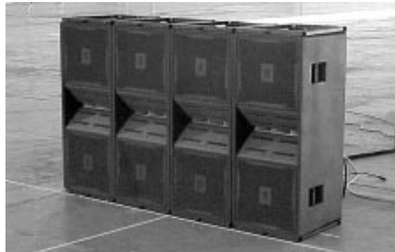
Four VT4889 enclosures set up for measurement sessions. Here, groundplane data is being gathered. The four boxes are set on end, at 0° splay angles.
