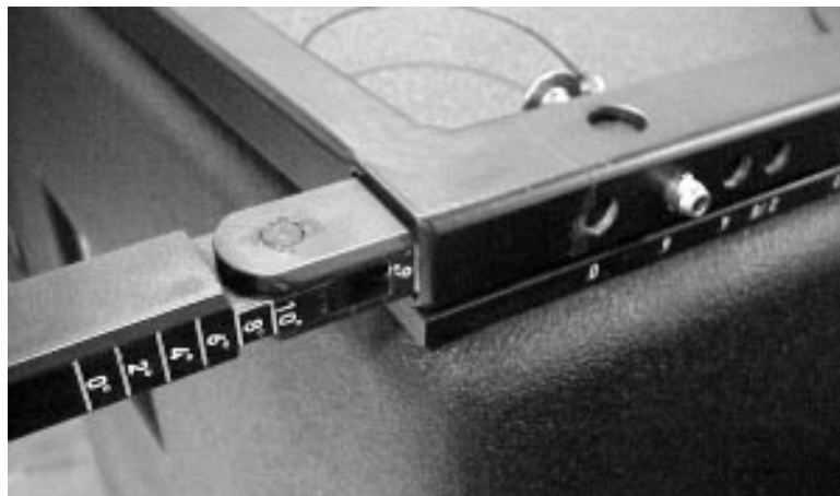
End corner view of a VT4889 enclosure showing the long (rear) hinge bar out of its storage channel, and pinned to the rigging frame. Note this bar is set in the six degree position.
