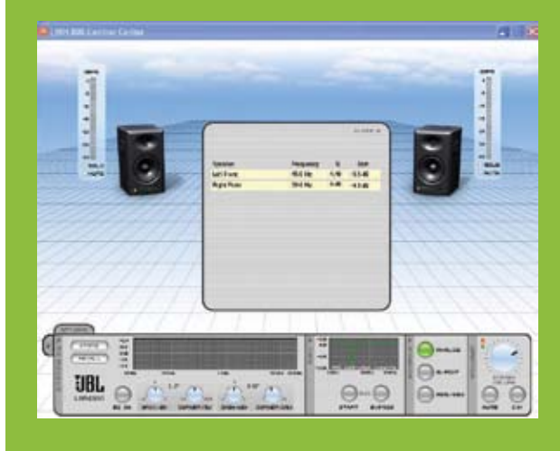
FIG. 3: The Control Center software gives you finer control over levels, input switching, EQ, muting, and more. It also displays the specific parameters of the RMC EQ curves (as shown here) that the system has generated.
