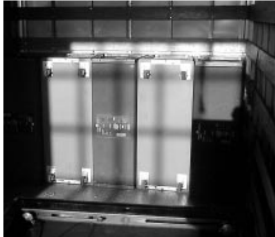
When enclosures are packed with fronts and backs alternating, rows of boxes take up less truck space.
