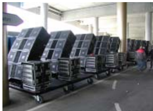
Line Array On-Ramp: JBL VERTEC VT4889 line arrays with Crown amplifier racks on custom carts from Sirius Showequipment a.g., ready for field deployment at the 18 th FIFA World Cup Opening Ceremony in Munich, Germany.
