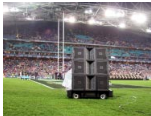
Powerful, lightweight JBL VT4889 line array modules were positioned on 18 custom mobile carts like this one by Jands Production Services to provide concert-quality audio for 85,000 persons at Australia's National League Grand Finals.
