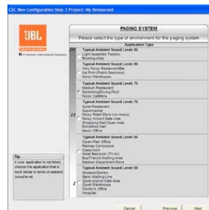
The JBL Professional CSC software identifies the appropriate JBL in-ceiling loudspeaker models and system design for any environment.
