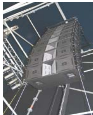
JBL VERTEC VT4888 midsize line array elements, supported by VT4880 fullsize subwoofers, were deployed by French audio rental firm Digiteac for this year's Festilac 2006 in Gene
