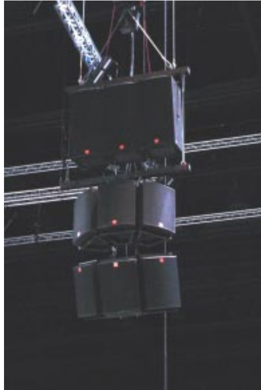
Mobile System Speaker Cluster Consisting of Venue Series and Sound Power
