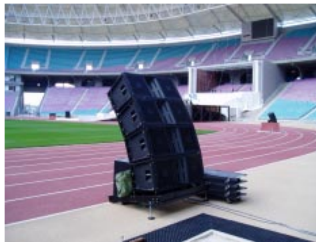
The sound reinforcement system for ACN 2004 (African Cup of Nations) included sixteen Crown-powered JBL VERTEC arrays. Each array featured four VT4889 line array elements, stacked for optimum coverage of the 65,000 seat stadium.
