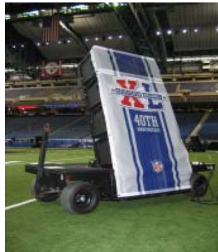
For Super Bowl XL, ATK/Audiotek is using their custom-designed cart system, loaded with JBL VERTEC loudspeakers, to provide full-range concert sound for the Rolling Stones.
